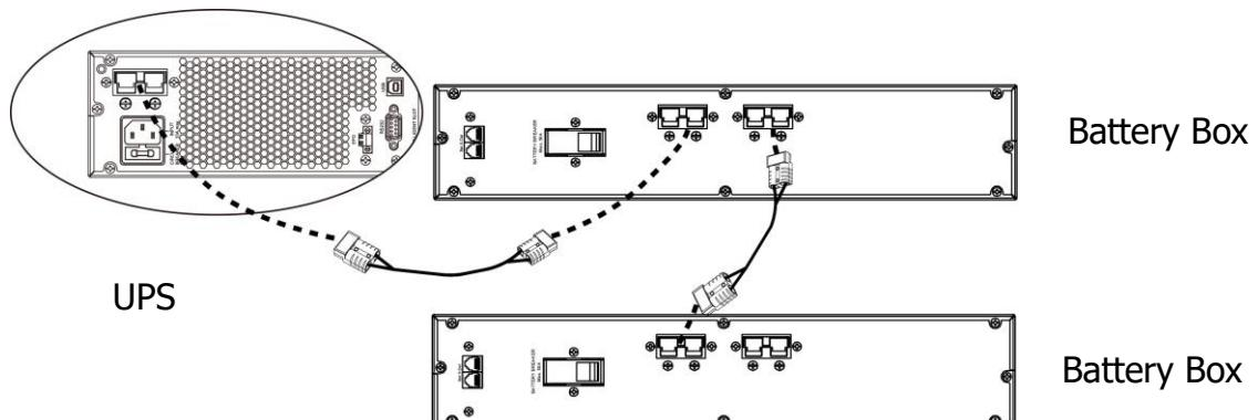
**NOTE:** If connecting more one external battery box, it's requested to connect load at 80% of UPS capacity.
