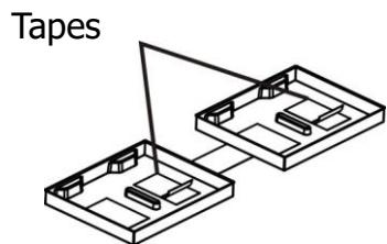
**Step 3:** Put assembled battery packs on one side of plastic shells.
