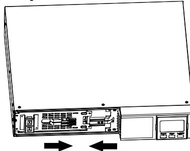
Connect the AC input and re-connect battery wires.
