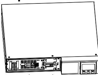
Disconnect battery wires.
