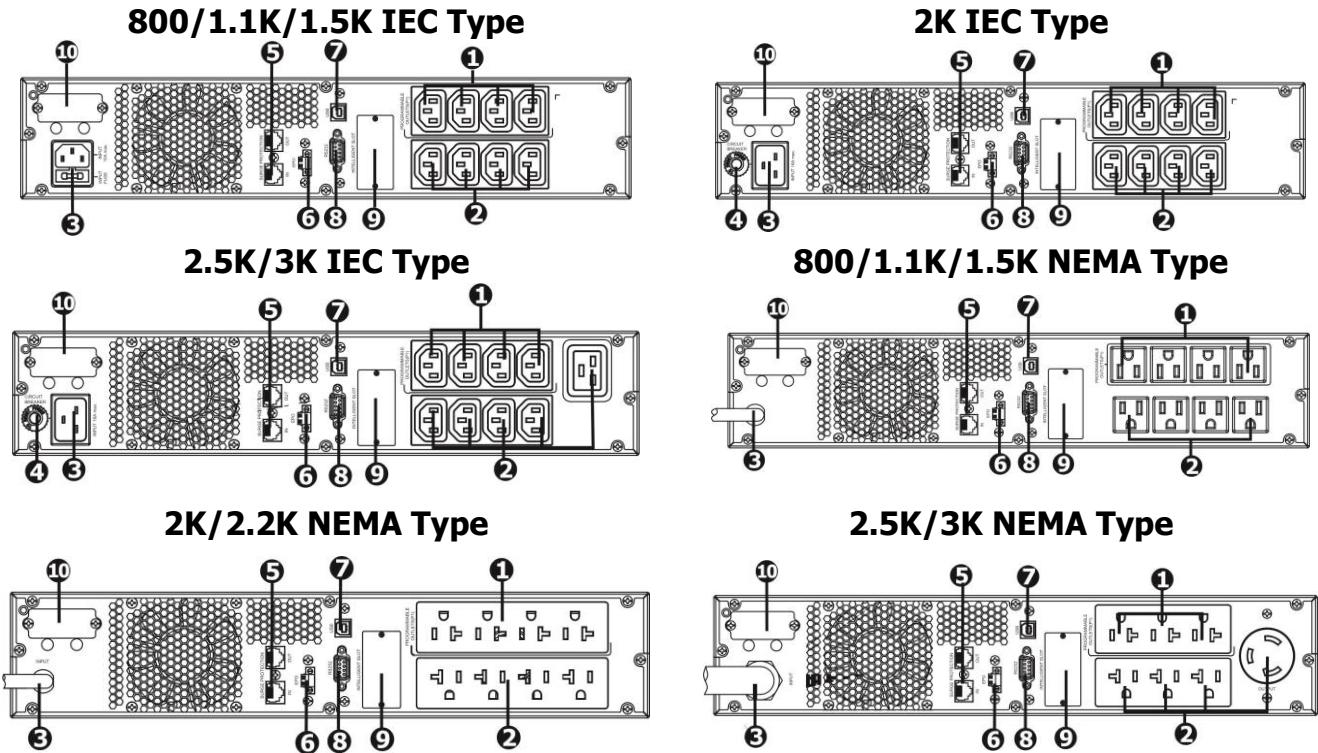
1. Programmable outlets: connect to non-critical loads.
