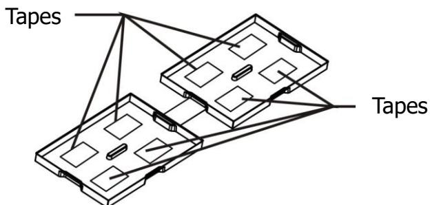
**Step 3:** Put assembled battery packs on one side of plastic shells.
