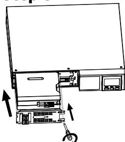
After replacing the batteries, put the battery box back to original location. Put the front panel back to the unit and install screws.
