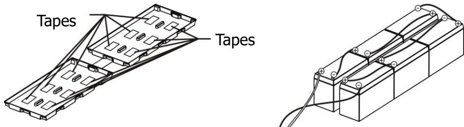
**Step 3:** Put assembled battery packs on one side of plastic shells.
