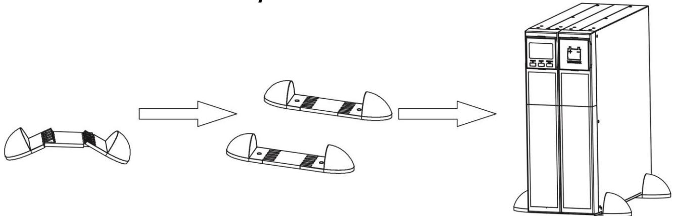
**NOTE:** When installing the UPS or battery pack with feet, please keep 70mm distance from the edge of the unit.
