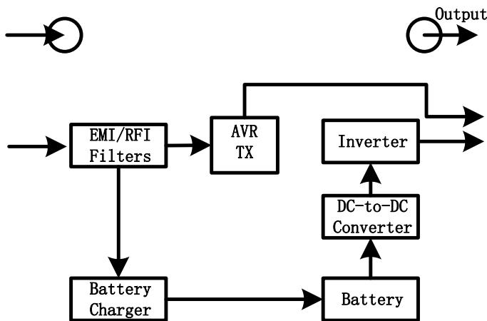
The UPS is composed of mains input, EMI/RFI Filters, Inverter, Battery charger, DC-to-DC converter, battery, AVR TX and UPS output
